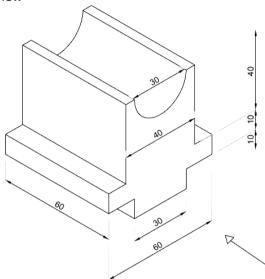
Q.7 The orthographic views of an object using first angle projection method are shown in figure. Draw its isometric view.
