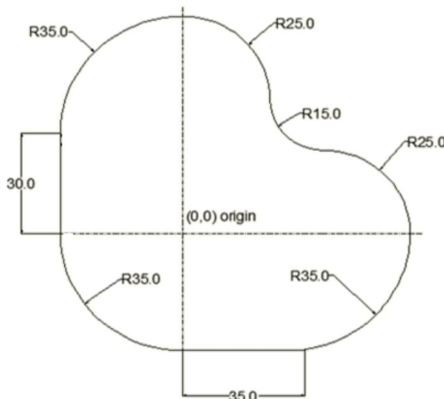
Fig 1( all dimensions are in mm, thickness 5mm)
