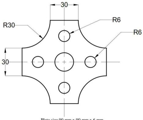
Plate size 90 mm x 90 mm x 6 mm All dimensions are in mm FIG.-2
